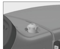
Fig.5.29 Diesel Tank Cap
