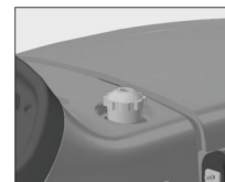
Fig.5.29 Diesel Tank Cap
